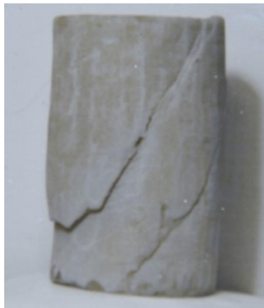
Figure 16. In a triaxial compression test, the hard mudstone specimen loses symmetry as a result of plastic strain softening.
